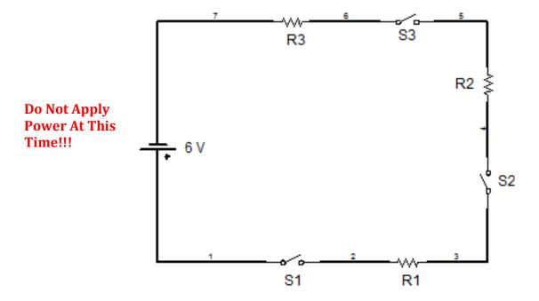
You should have (7) total wires when completed. Please have your instructor verify the correct wiring of the circuit before proceeding!
